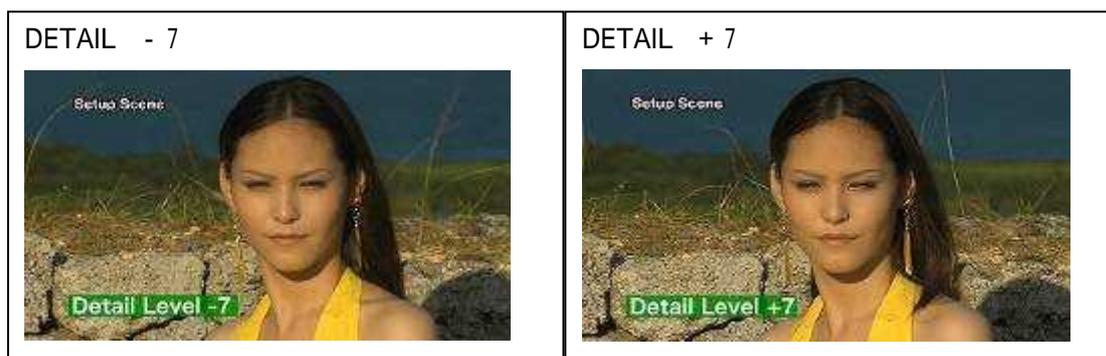
AG-AC160 is equipped with two DETAIL controls. One is for both the horizontal and vertical directions ("DETAIL LEVEL"). The other is for the vertical direction ("V DETAIL LEVEL"). Balance of horizontal and vertical detail effects can be adjusted by these two controls within a certain range of edge signals.
